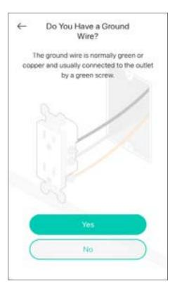
At least one black wire and one white wire should be connected to your old outlet. If you have additional or different colors, alternative wiring steps may be necessary.
