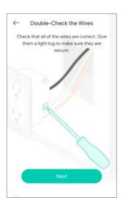
Notice: For the sake of safety, the naked part of the wire should not be too long. Wires extending out the Smart Outlet should have sufficient insulation.
