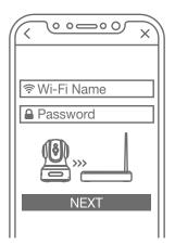
NOTE: Place smartphone and camera as close to the router as possible. The encoded sound will be audible through your smartphone speaker during connection process.
