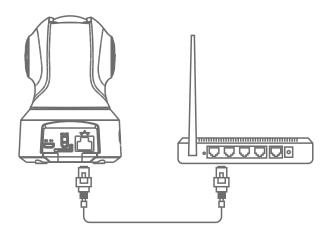
**2.** Tap Ethernet Connection icon button. Wait until camera is connected. Change password and set Wi-Fi (Optional).
